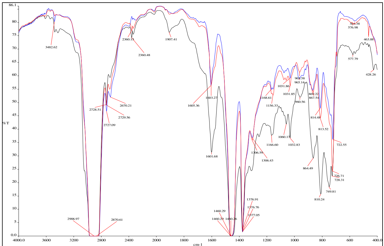
Fig.-7: FTIR of oils: Black color high PCA/ Blue color Oil No1/ Red color Oil 2
