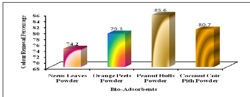
Fig-7: Maximum Colour Removal Percentage by Different Bio-Adsorbents
