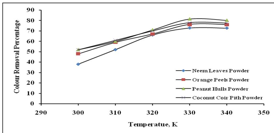
Fig.-5: Effect of Temperature on Colour Removal
