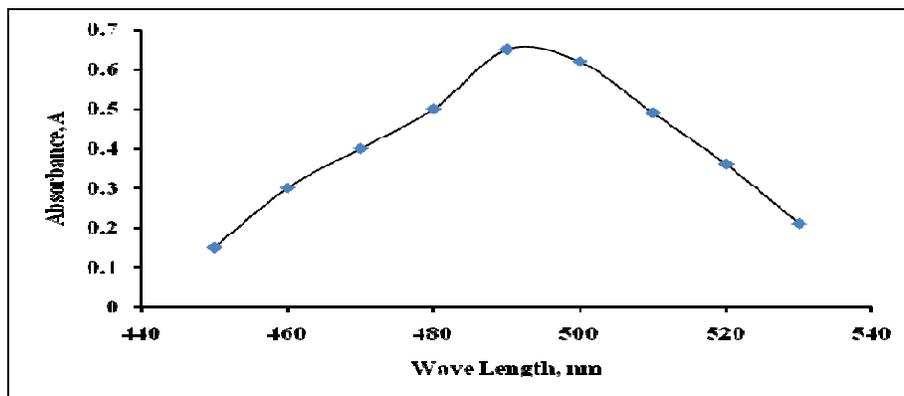
Fig.-1: Absorbance Curve for Textile Industry Wastewater
