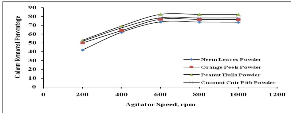
Fig-6: Effect of Agitator Speed on Colour Removal
