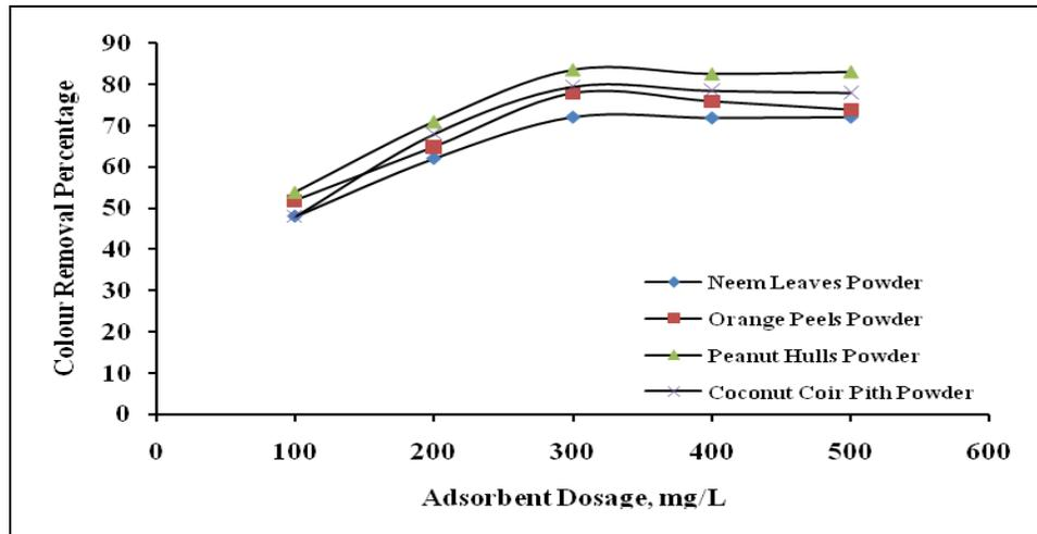
Fig.-3: Effect of Adsorbent Dosage on Colour Removal
