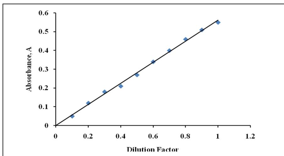
Fig.-2: Calibration Curve for Textile Industry Wastewater at a Wave Length of 495 nm
