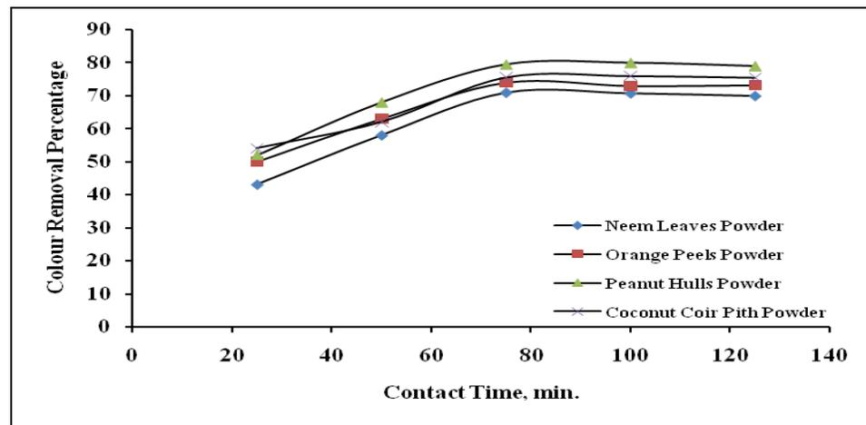
Fig.-4: Effect of Contact Time on Colour Removal
