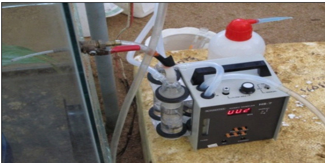
Fig.-2: Formaldehyde sampling from the experimental chambers
