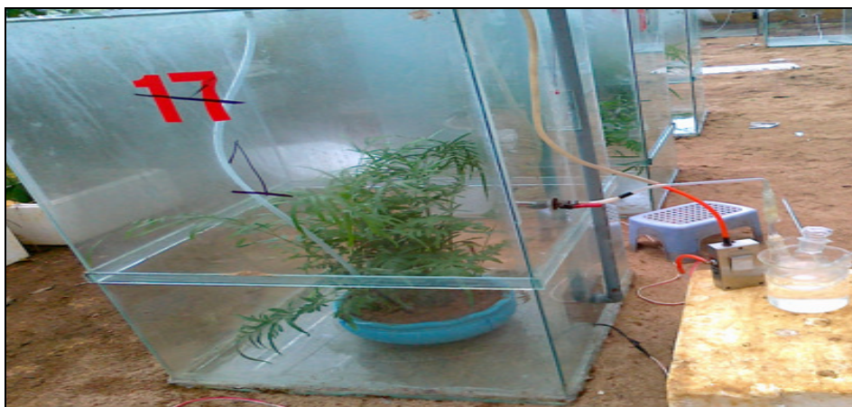
Fig.-1: Formaldehyde transfer to the experimental chambers.
